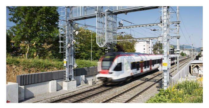
Numerous data and information are taken when trains pass train-monitoring installations. RFID technology now permits a more precise and reliable assignment of the gathered data to individual train cars and axles. Moreover, the relevant data can also be used for other applications. The aim of the present project is to assess the benefits of equipping wayside train monitoring installations with RFID technology.
