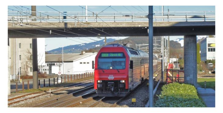
It may be necessary to analyze the collision risk for structures near railway lines. The aim of such analyses is to determine whether the risk of collision is acceptable or whether additional safety measures need to be taken.
