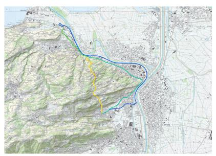
Comparison developed with the routing prototype showing the shortest (yellow), most energy efficient (turquoise) and fastest (blue) routes for private motor vehicle traffic.
