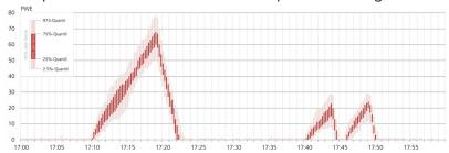
Legend: Queue lengths in Uznach during peak evening hours for traffic heading to Tuggen (delay scenario)
