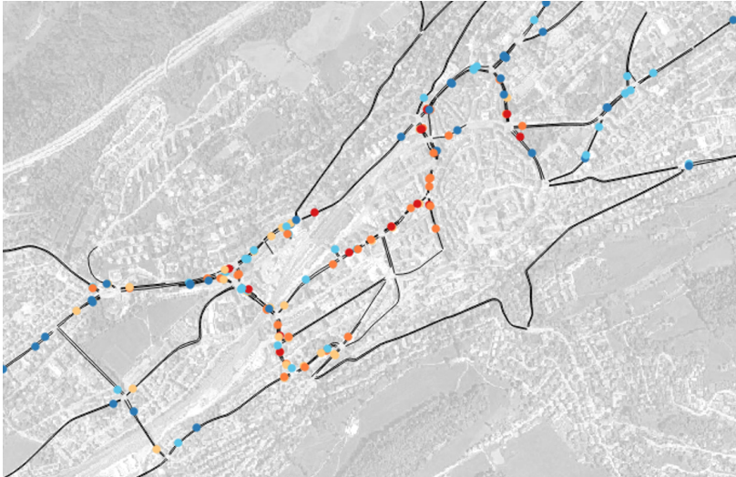
Representation of traffic states at the main nodes and segments in St.Gallen (red: low speed, blue: high speed)
