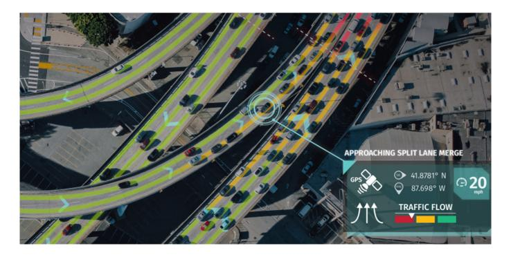
One essential benefit of new transport infrastructures is savings in travel time. For the Canton of Lucerne we compared travel times in the transportation model to travel times based on floating car data supplied by our partner HERE Technologies. Based on this, we calibrated the transportation model and determined correction factors. This allows us to ensure that our infrastructure-project assessments reflect reliable travel time and congestion level data.
