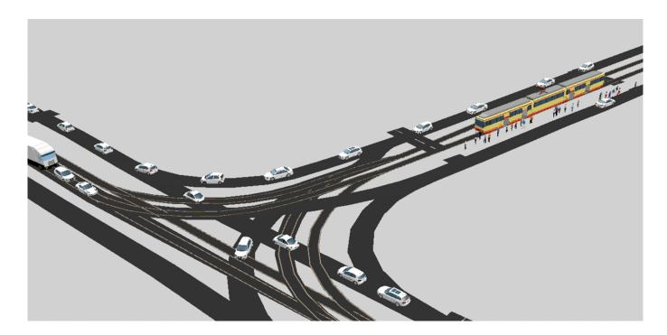
EBP has used traffic flow simulation to verify the capacity of a redesigned Rämistrasse-Gloriastrasse intersection to handle the anticipated traffic volume. The intersection is to be redesigned in the context of the further development of Zurich's university district.
